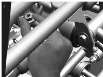
Fig. 12 Confirmation of workability (confirmation of working space)
