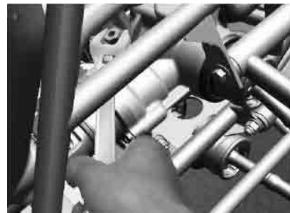
Fig. 13 Confirmation of workability (confirmation of tool interference)
