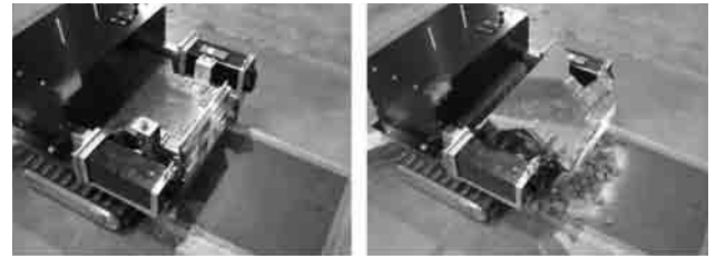
Fig. 8 Emission mechanism of rubble
