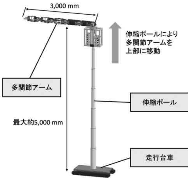
Fig. 9 Concept of a high place working equipment
