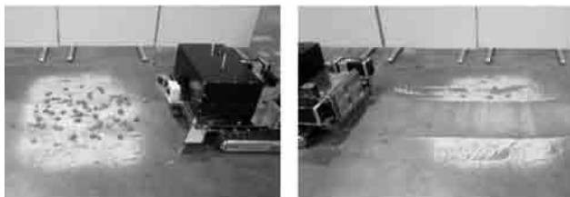
Fig. 7 Before and after collection of rubble
