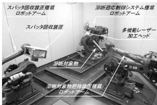
Fig. 16 Cooperative robot movement and adaptive laser cutting control system
